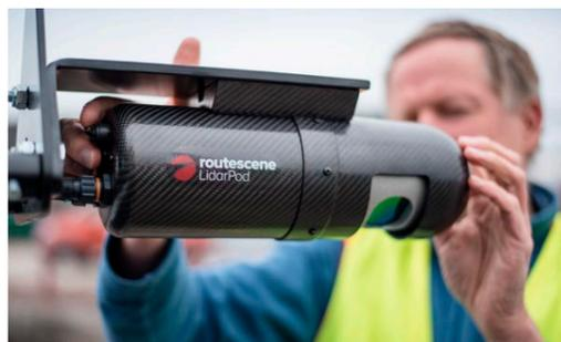
▲ Figure 4, Example of a turnkey mini-grade Lidar system developed by RouteScene that utilises a Velodyne HDL-32E scanner (photo: www.routescene.com).
