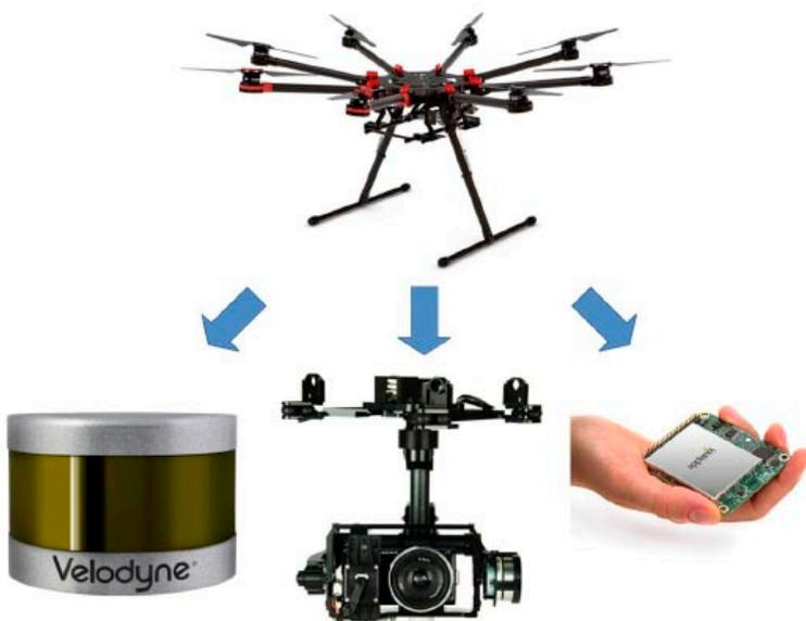
◀ Figure 2, Mini-grade UAS Lidar system being developed by researchers at Texas A&M University-Corpus Christi that integrates a DJI S1000+ platform with a Velodyne VLP-16 Lidar scanner. The system will use an Applanix APX-15 high-accuracy INS (weighing 60 grams) and employ a Zenmuse Gimbal Z-15 for mounting a Sony Alpha Nex 7 camera.
