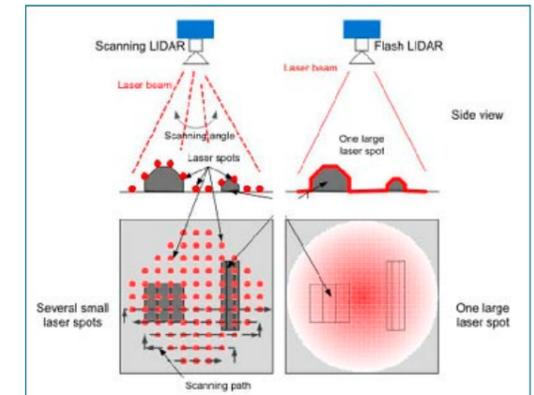
▲ Figure 6, Scanning Lidar compared to flash Lidar (photo: adapted from www.fosternav.net).
