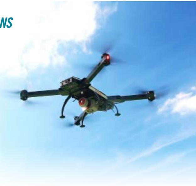
◀ Figure 1, RIEGL VUX-1 mounted on the RiCOPTER platform (photo: www.rieglusa.com).
