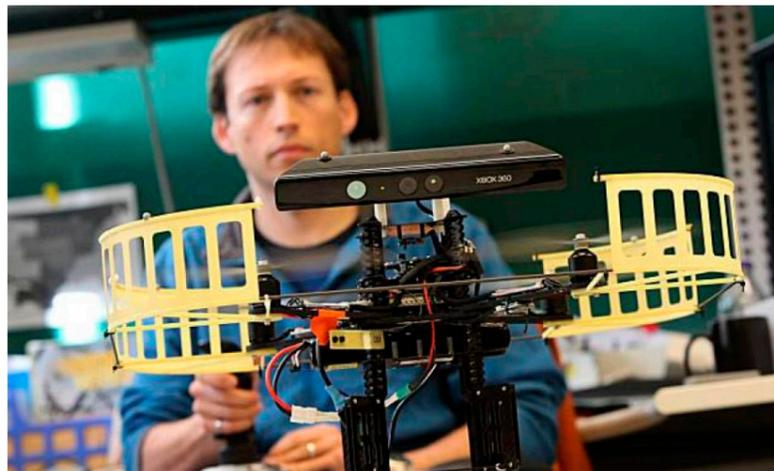
▲ Figure 5, Micro-grade UAS equipped with Xbox Kinect for autonomous flight developed by researchers at University of California, Berkeley, back in 2010 (photo: Liz Hafalia, The Chronicle).
